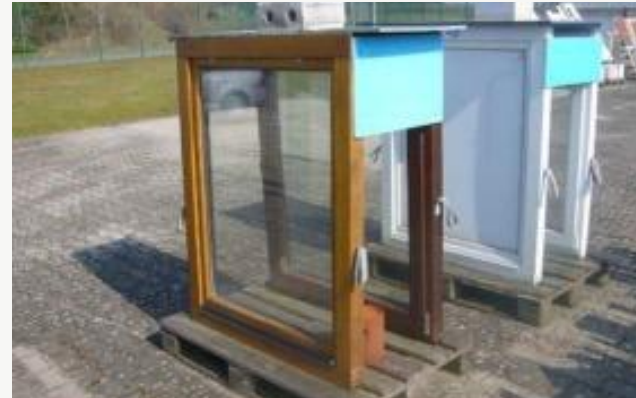
No coating degradation visible after 14 years
